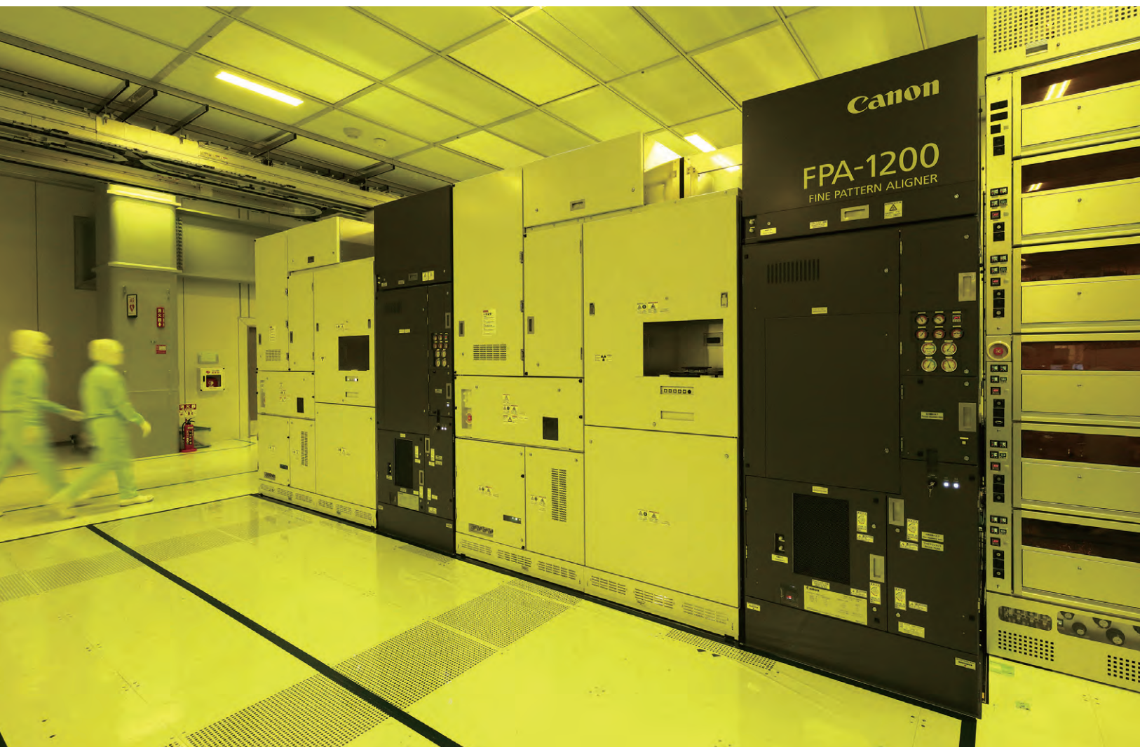
Nanoimprint lithography can significantly reduce manufacturing costs and power usage
